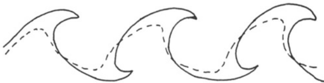
FIGURE 27. Comparative interface visualization of the two vorticity modes (near-side views). (a) Non-symmetric one resulting from the vertical perturbation. Corrugated splitter plate. (b) Symmetric one resulting from the horizontal perturbation. Indented splitter plate. The cross-sections A-A and B-B are in the two cases a half wavelength apart.
